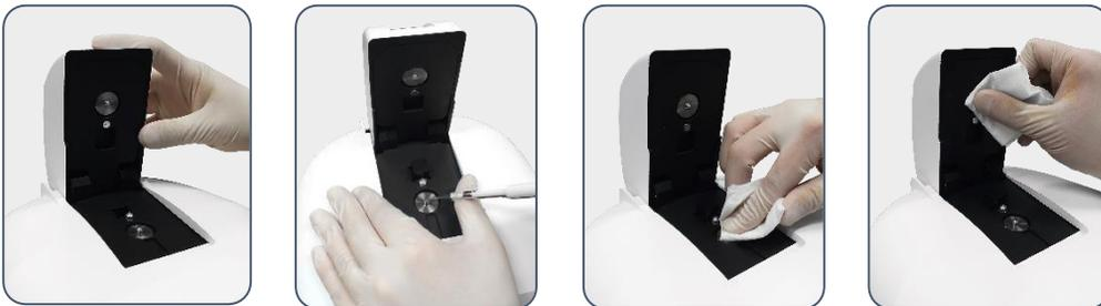
Microvolume sample measurements include the use of the Pedestal.
